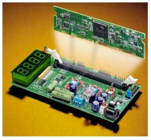
Connect the J1 connector of the board to the JTAG emulator, and then connect the JTAG emulator to the computer's USB port. After connecting the power to the board, turn on Switches SW1 and SW2 on the board. Switch SW3 is for displaying either Ch1 or Ch2 output. Set SW3 to the Ch2 position.
