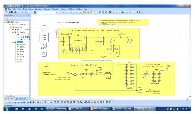
As compared to a circuit not for code generation, this circuit contains elements from the F2833x Target library. In this circuit, there are two F2833x Target library elements: a 16-channel A/D converter and a 1-phase PWM Generator, as shown below on the left.
