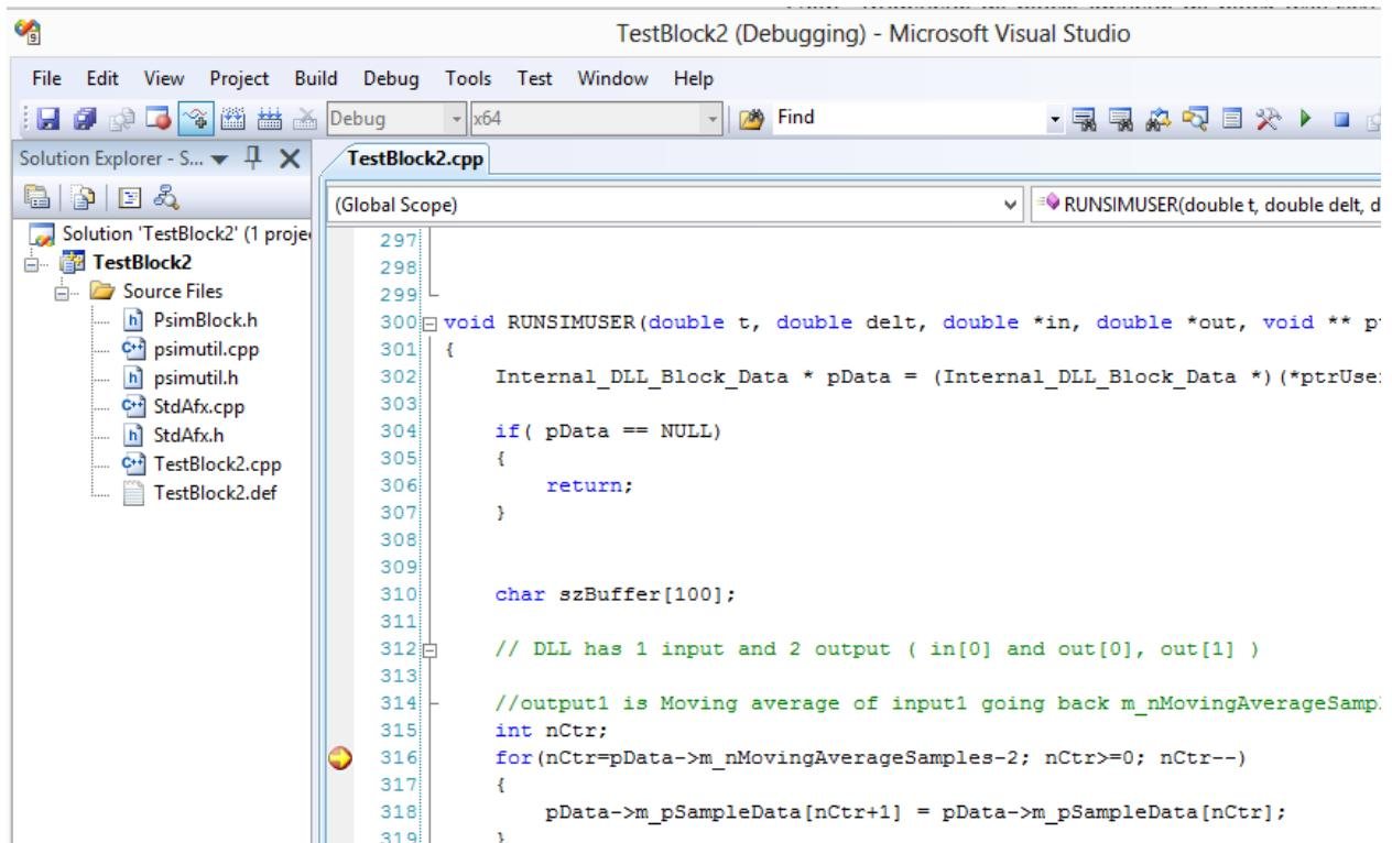
If execution does not stop, check the location of the break points. One common error is that a wrong DLL file, or the release version of the DLL file, is selected for the general DLL block. The path of the generated DLL file is shown in Visual C++ as shown below.
